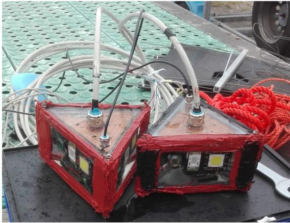
Figure 7. ENEA's proof-of-concept optical modem.
